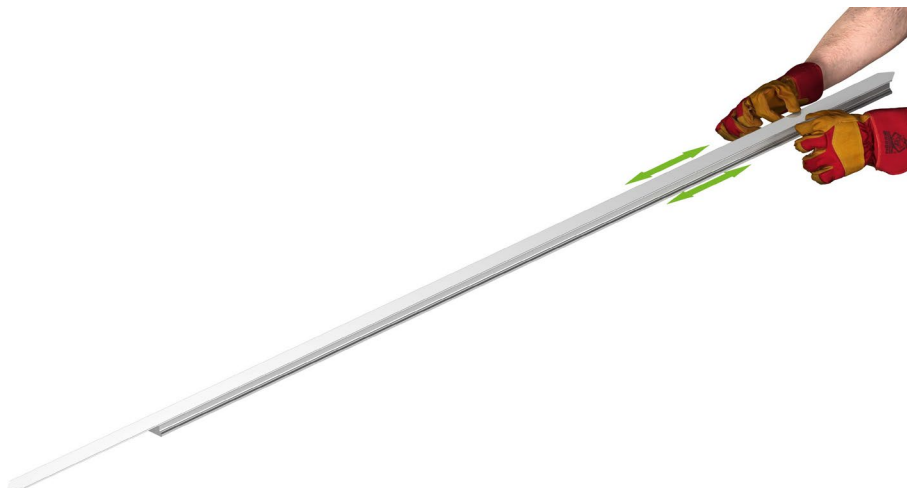
Fig. 5.28: Clamp on cover strip approx. 3 cm
