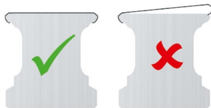
Fig. 5.45: Correctly and incorrectly fitted cover strip
